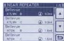
Display example of IC-7100 (Shows near repeater list with distance)
